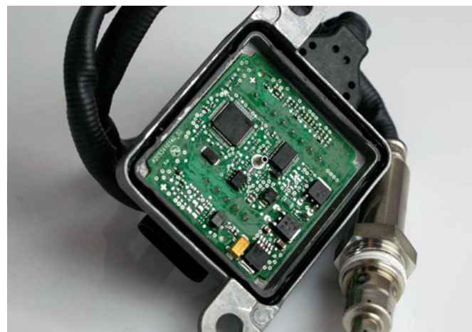
Figure 3. Sensor circuit board
