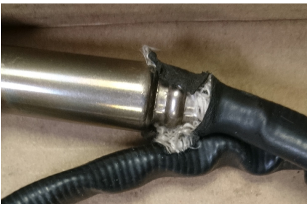
Figure 14. Evidence of damaged wiring.
