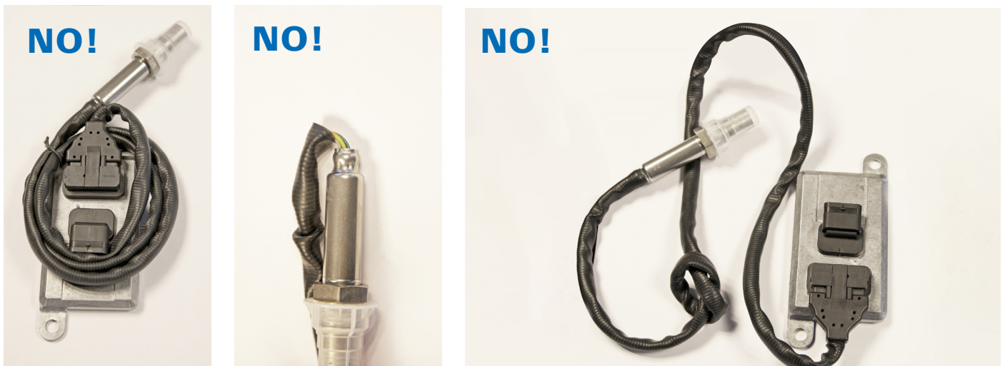
Figure 5. Inappropriate wire handling.
