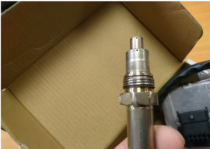
Figure 11. Damaged sensor thread and nut.
